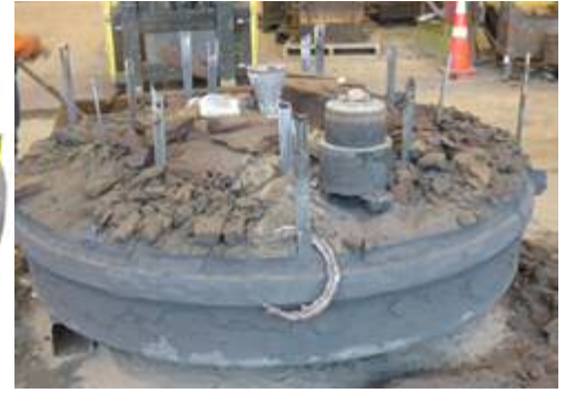
FIGURE 4: Single riser design. Casting Model (left), Shop Floor (right)
